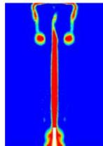
within ANSYS Fluent, a jet impinging onto a flat plate is modeled as a transient, two-phase flow. The results of simulations that examine the effects of nozzle velocity and temperature on the jet flow profiles and impingement area will be reported. Such results are expected to contribute to the development of heat transfer correlations for oil-jet cooling applications.
